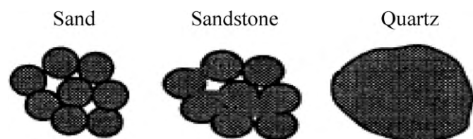
Fig. 2. Schematic diagrams showing the evolution of the porous structure during the diagenesis of quartz. As diagenesis progresses, sand grains become compacted and cemented. The initial porosity (40%) decreases down to zero. Modified after ref. [63].
